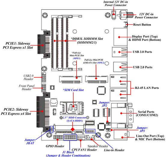
Note: 1.The memory module should be DDR3L 1.35V SODIMM and not exceeding 16GB total capacity. 2. SIM card slot only work when compatible SIM card installed & 3G LAN card installed in MPE1 Mini-PCIE slot.
