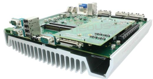
Neousys provides various MeziO™ modules, such as RS-232/422/485, isolated DIO, LVDS output, CAN bus, ignition power control, and DTIO, as the options for Nuvo-5000. Users can also leverage signals/powers on MeziO™ to create a module with specific domain know-how. MeziO™ presents a cost-effective way to build a tailor-made embedded system for your application.
